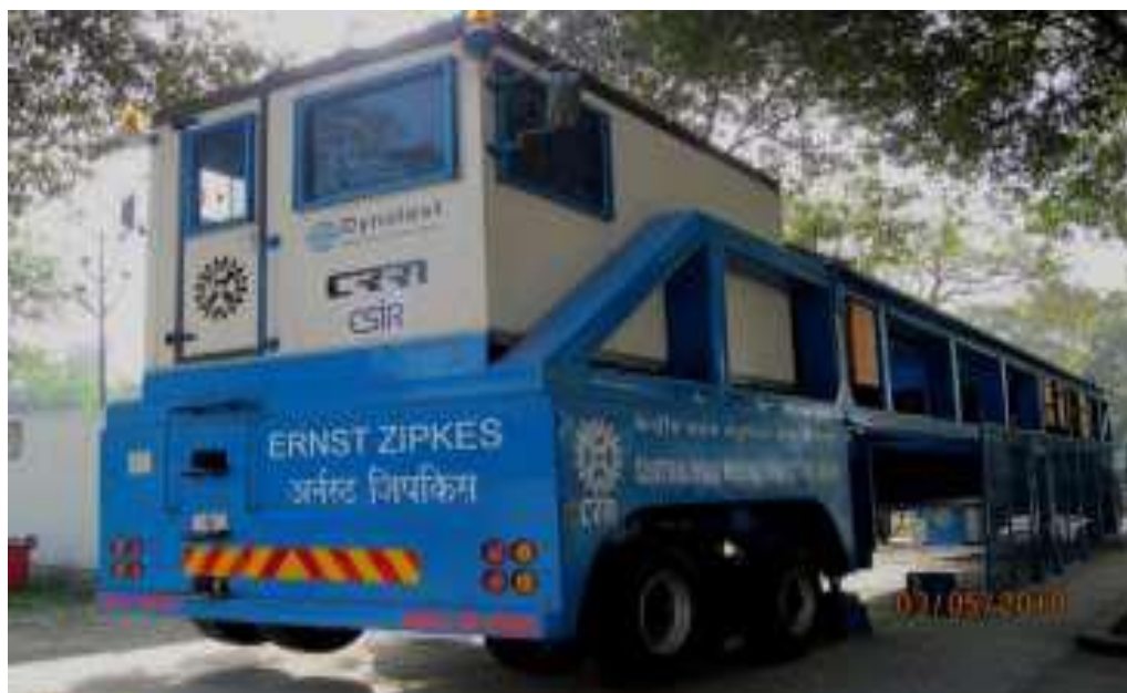
Figure 3: Accelerated Pavement Testing Facility to be used for evaluation of proposed designs of roads
