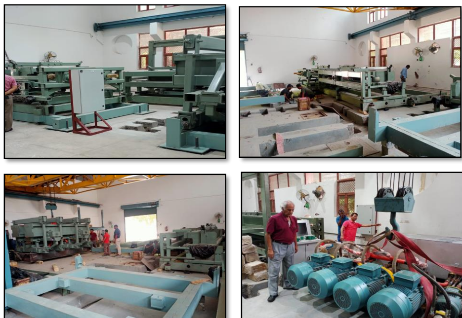
Figure 11: Showing the Installation of Test Rigs and Power Pack in Progress
