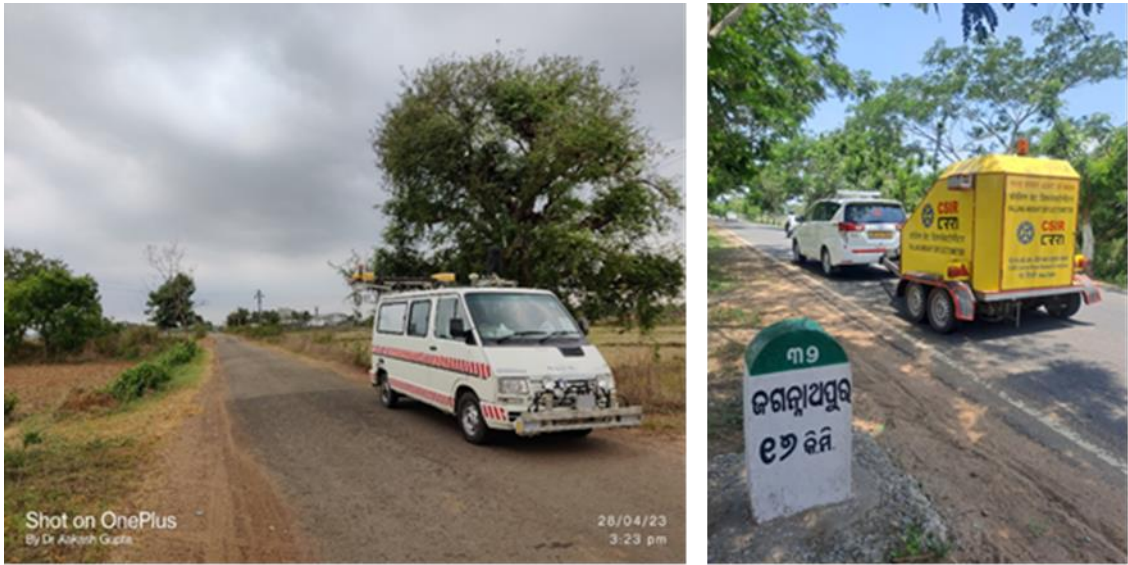
Figure 9: NSV and FWD Surveys on Project Roads in Odisha
