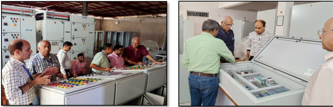
Figure 12: Showing PDI of PKG2 Electrical Panels and PDI of PKG-3 Control Panels
