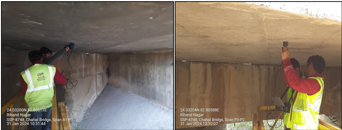
Figure 26: A Typical View of Non-Destructive Testing of the Deck Slab of Span A1-P1 and P2-P3 of Chahal Bridge of the NTPC at Rihand.
