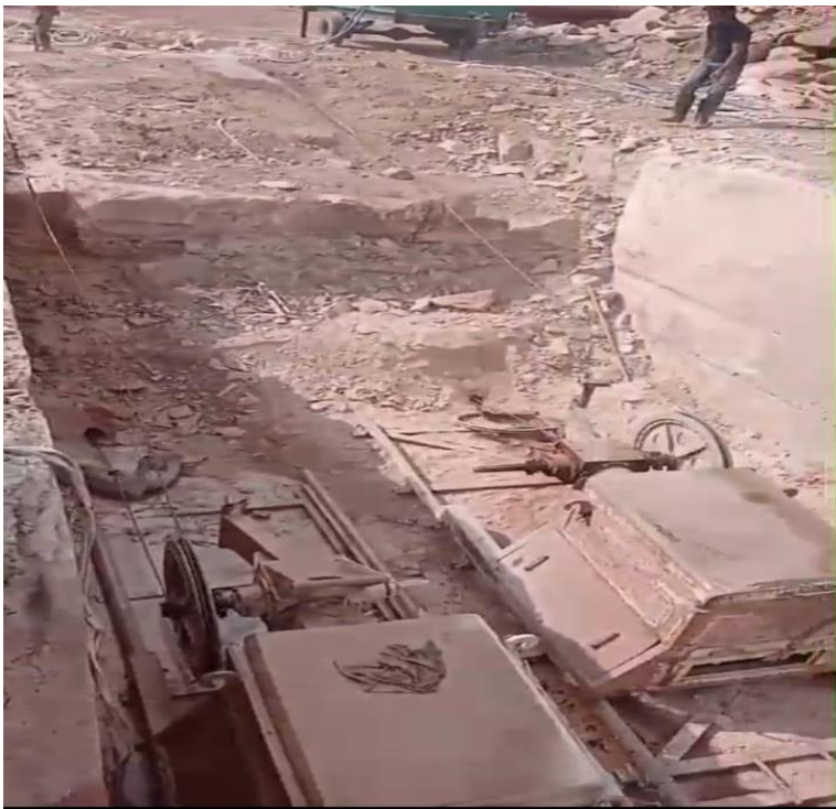
Figure 3: Recommended Diamond Rock Cutting method for the protection of Chandpur-Jhansi ancient monuments from vibration
