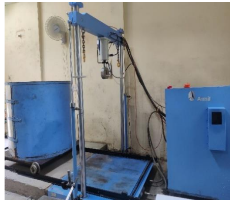
Figure 4: Cyclic plate load test on reinforced and unreinforced model pavement layers
