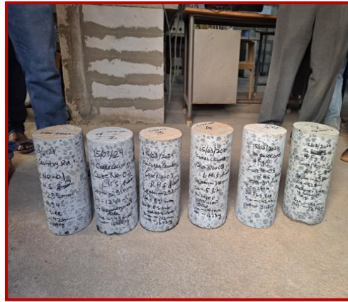
Fig 12. Extract concrete core from the test tracks
