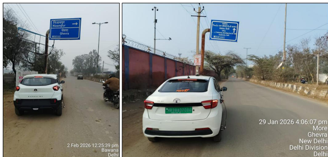
Photo 16: IRI survey using Roughometer III equipped within EV
