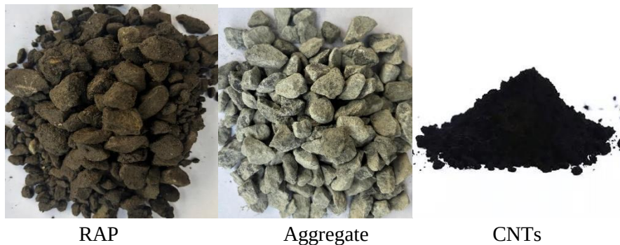
Photo 28: Ingredients of Concrete used and prepared Specimens
