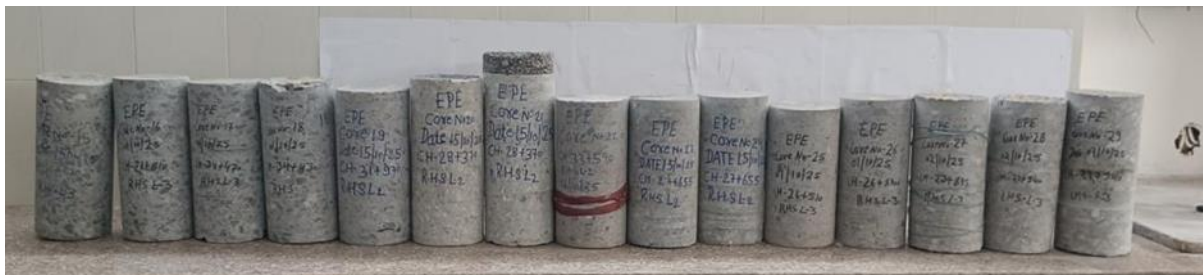
Photo 26: Extracted PQC core samples
