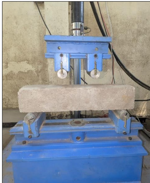
Photo 6: Flexural Jig for Fatigue Test
