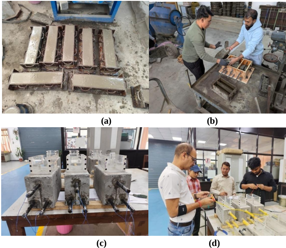
Photo 2: (a) View of beams cast to measure the Flexural Strength (b) Casting of specimen for measurement of Corrosion Effect as per ASTM G 109. (c) Plastic pond installed on the top of the specimen to store sodium chloride (d) Measurement of Corrosion Potential is under process (first reading).
