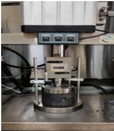
Figure 3: Dynamic Creep test for long-term deformation behaviour under repeated loading
