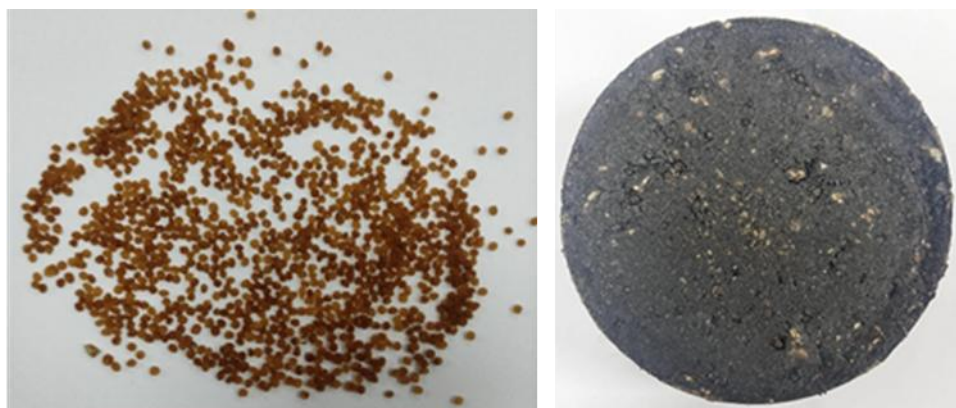
Figure 6: Microcapsule Encapsulated Rejuvenators (left) and Microcapsule embedded compacted asphalt mix (right)
