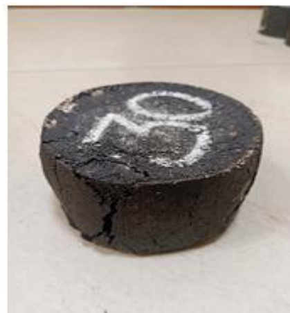
Figure 3: Dynamic Creep test for long-term deformation behaviour under repeated loading
