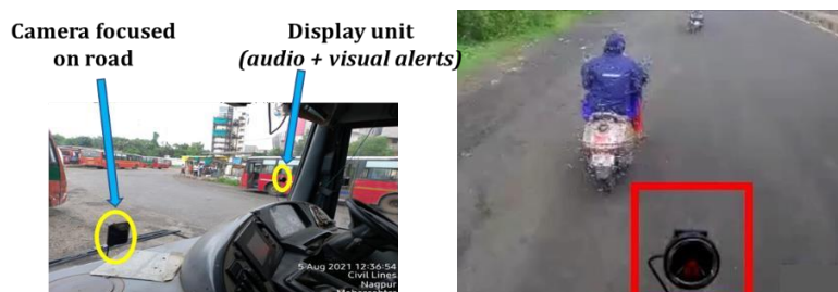
Figure 3: CAS unit installed in a bus; Typical Illustration of PCW warning generated due
