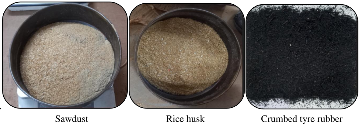
Figure 8: Three Types of Infilled Materials used in Trench Wave Barriers for Vibration Screening
