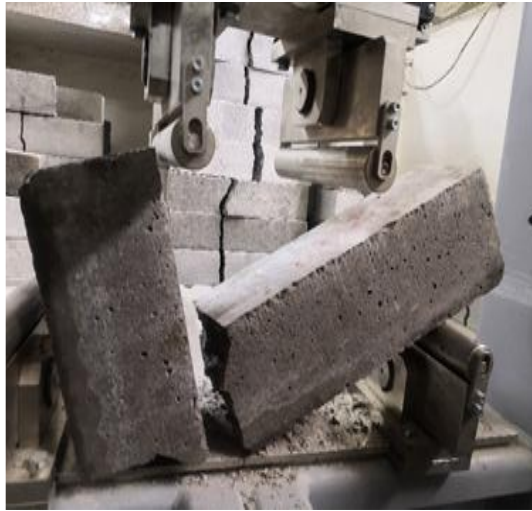
Figure 2: Flexural strength test
