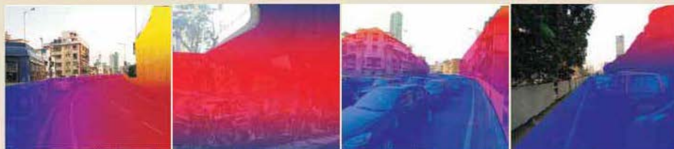
Fig.4 : Noise Mapping (Top/Bottom of JJ Flyover) showing the affected area with different noise levels
