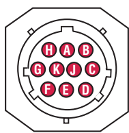
Male, 10-pin in-line or integral MS connector (Option FM_ or MSO)
