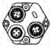
Figure 1. R-Series sensor Integrated diagnostic LEDs
